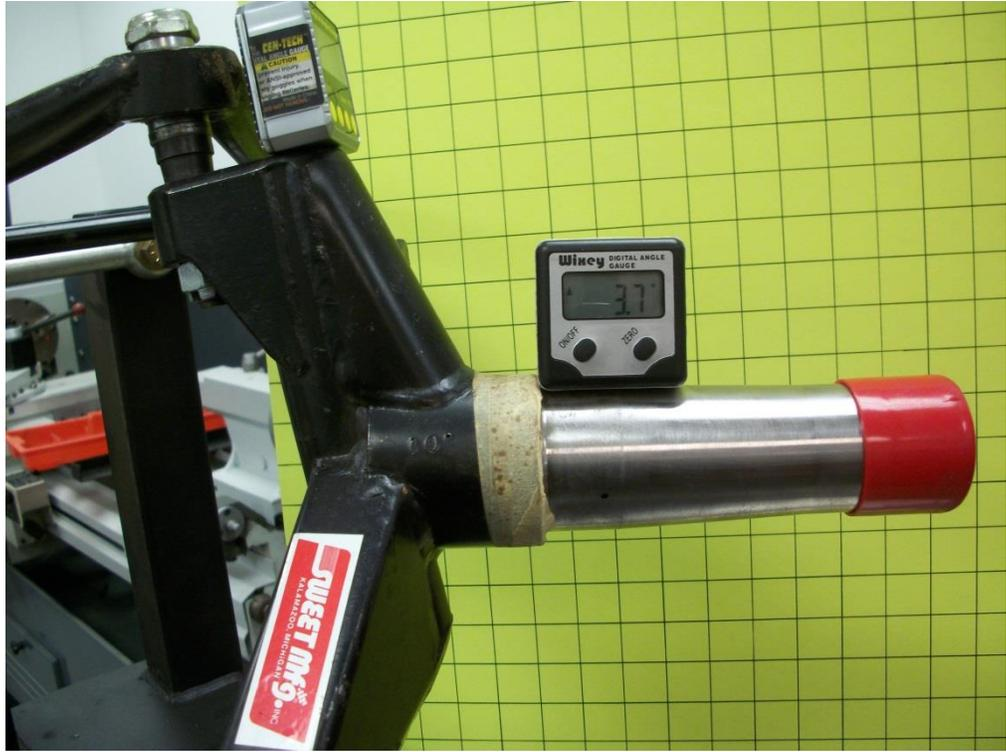
Figure 7: Same spindle as above with the wheel steered approximately 30 degrees (just to show effect) showing camber change. Note camber is now positive (out at the top).
