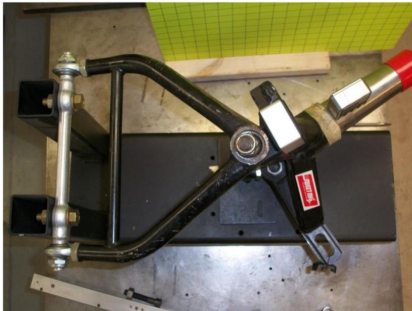
**Figure 12:** A top view to show the steering angle where camber returned to the original 1 degree as the wheel was turned left with a 5 degree caster setting.
