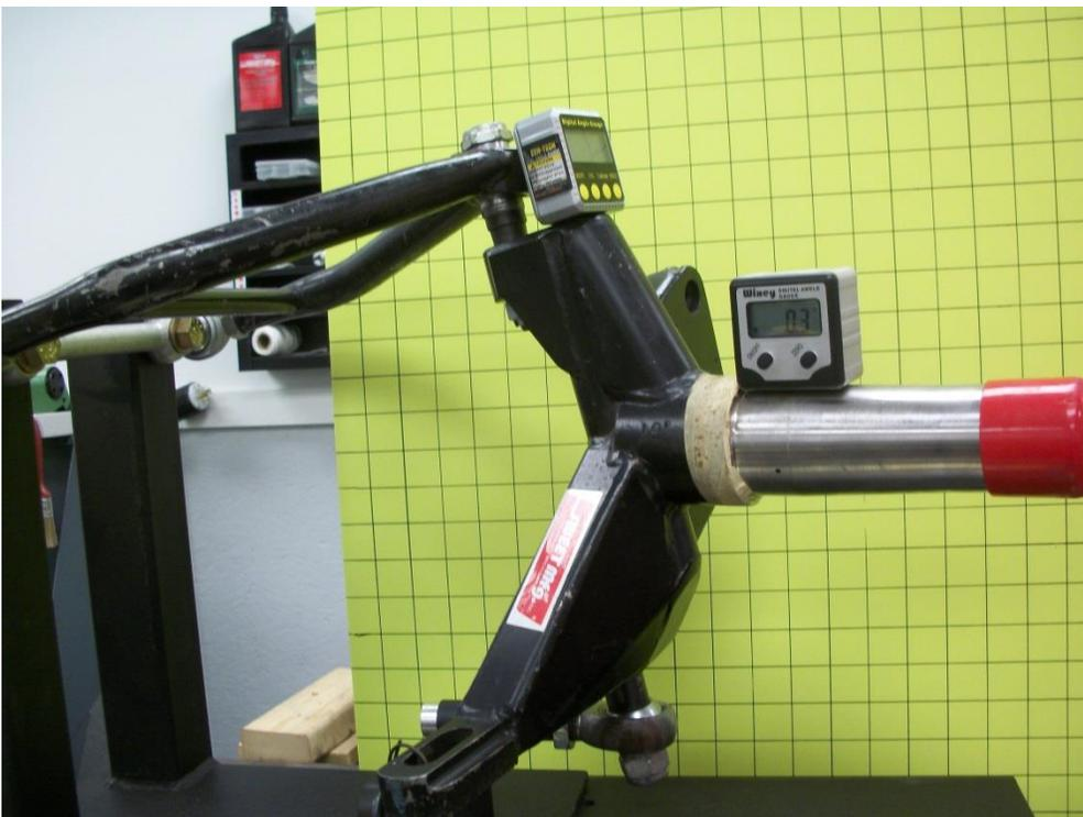
Figure 9: Same spindle as above caster=0, initial camber=1 negative, steered 10 degrees to right, camber now showing 0.3 degrees (still negative) it lost 1.0-.3 or .7 degrees in steering.
