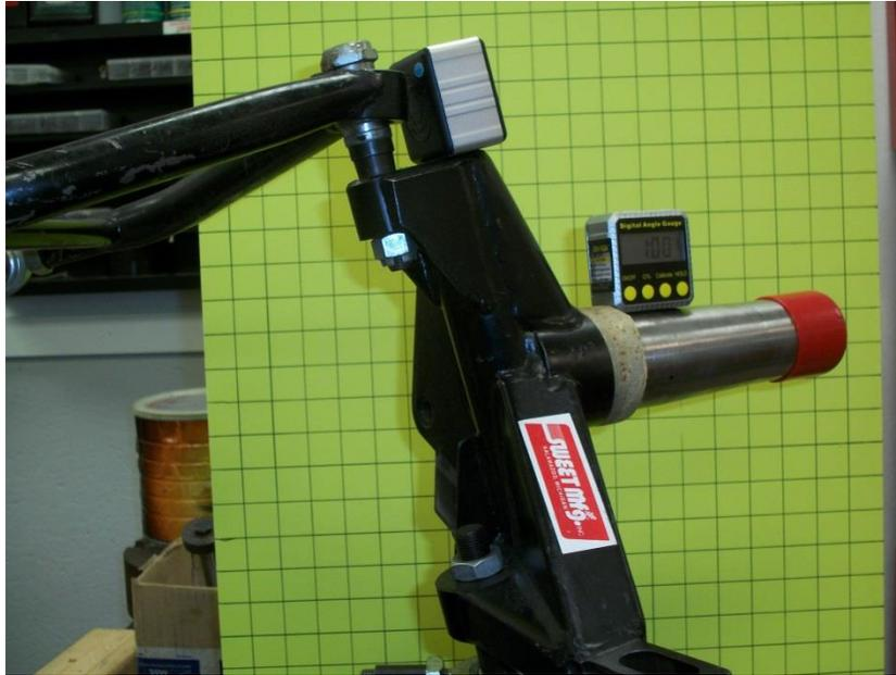
**Figure 11:** A 10 degree spindle with caster = 5 degrees positive, static camber = 1 degree negative and turned to the inside until the camber reached 1 degree negative (the static setting)
