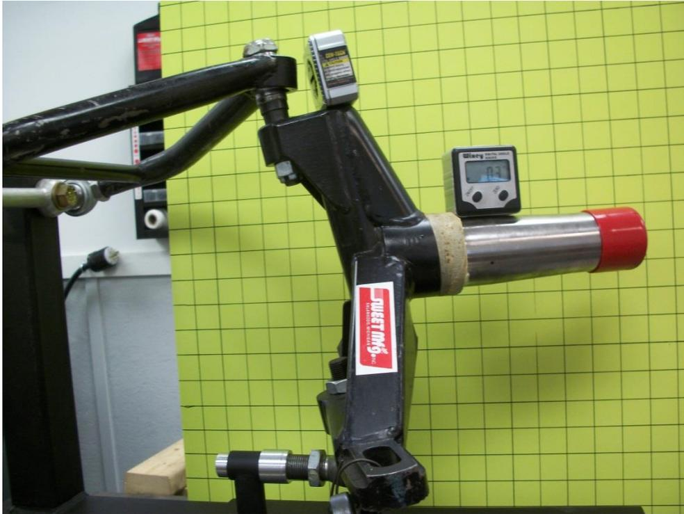
Figure 8: Same spindle as above caster=0, initial camber=1 negative, steered 10 degrees to left, camber now showing 0.3 degrees (although still negative) it lost 1.0-.3 or .7 degrees in steering.
