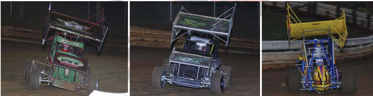
Here you can see in these three pictures the cars are all winged left and transferring weight to the left side of the car in corner entry.
