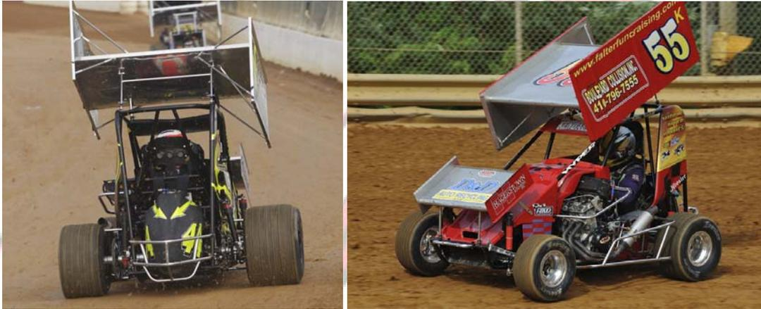
You can see in the above pictures that the cars are now transferring weight to the right side of the car in the rolled right phase on corner exit. Interesting too you can see in Robie's 55 car, the left front shock is topped out and just about off the ground, all the weight that was on the left front has now mostly transferred to the right rear and right front, He can still steer off the right front, so this is not a bad thing.
